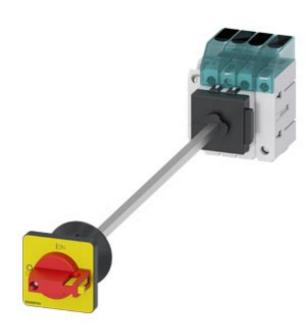
Switch disconnector 3LD3, main switch 3-polig + N, lu 25A operational switch at AC-23 A at 400 V 9,0 kW floor mounting Base mounting with door coupling center-hole 22,5 mm knob-operated mechanism red/yellow 48 x 48 mm with auxiliary 1NO+1NC
