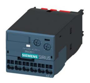
SOLID-STATE TIME RELAY ON-DELAY WITH SEMICONDUCTOR OUTPUT 24...240V AC/DC TIME RANGE 0.05...100S FOR SNAPPING ONTO THE FRONT; FOR 3RT2 CONTACTORS S00/S0 SPRING-TYPE TERMINALS INTEGRATED VARISTOR FOR DAMPING CONTACTOR COILS
