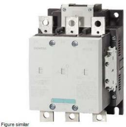
VAC. CONTACTOR, 160KW/400V/AC-3 AC(40...60HZ)/DC OPERATION UC 500-550V AUXILIARY CONTACTS 2NO+2NC 3-POLE, SIZE S10 BAR CONNECTIONS CONVENT. OPERATING MECHANISM
