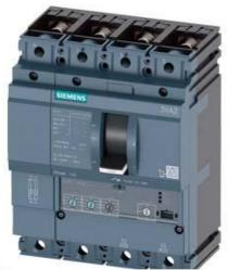
CIRCUIT BREAKER 3VA2 IEC FRAME 100 BREAKING CAPACITY CLASS L ICU=150KA @ 415 V 4POLE, LINE PROTECTION ETU320, LI, IN=63A OVERLOAD PROTECTION IR=25A ...63A SHORT CIRCUIT PROTECTION II=12 X IN NEUTRAL PROTECTION ADJUSTABLE(OFF,100%) BUSBAR CONNECTION
