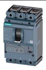
CIRCUIT BREAKER 3VA2 IEC FRAME 160 BREAKING CAPACITY CLASS L ICU=150KA @ 415 V 3POLE, LINE PROTECTION ETU350, LSI, IN=160A OVERLOAD PROTECTION IR=64A ...160A SHORT CIRCUIT PROTECTION ISD=1,5... 10 X IR, II=10 X IN CABLE CONNECTION
