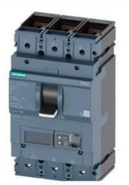
CIRCUIT BREAKER 3VA2 IEC FRAME 630 BREAKING CAPACITY CLASS M ICU=55KA @ 415 V 3-POLE, LINE PROTECTION ETU550, LSI, IN=500A OVERLOAD PROTECTION IR=200A ...500A SHORT CIRCUIT PROTECTION ISD=0,6..10X IN, II=1,5..14X IN NEUTRAL PROTECTION OPTIONAL WITH EXT. CT;UPTO 160% BUSBAR CONNECTION
