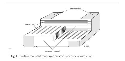
Surface-Mount Ceramic Multilayer Capacitors Y5V SERIES 6.3 V to 50 V
