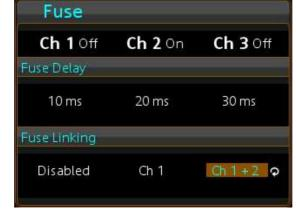
Users can set the power supply so that all channels are switched off if one channel hits the limit. Or it can be set to leave one channel working.
