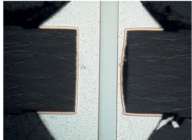
Microsection of R-TECH SAC alloy, showing a good even fill and even with poor pin placement.
