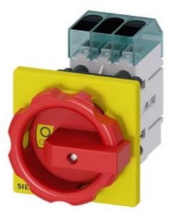
Switch disconnector 3LD3, main switch 3-polig, Iu 16A operational switch at AC-23 A at 400 V 7,5 kW front mounted Base mounting with center-hole 22,5 mm rotary operationg mechanism red/yellow 66 x66 mm
