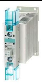
SEMI-COND. CONTACTOR 3RF2,1-PH. AC 51 30 A 40 DEGREES C 48-460 V / 110-230 V AC RING TERMINAL
