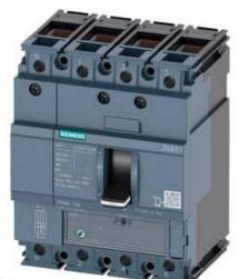
CIRCUIT BREAKER 3VA1 IEC FRAME 160 BREAKING CAPACITY CLASS N ICU=25KA @ 415 V 4-POLE, LINE PROTECTION TM220, ATFM, IN=125A OVERLOAD PROTECTION IR=87,5A ... 125A SHORT CIRCUIT PROTECTION II=10 X IN NEUTRAL UNPROTECTED CABLE CONNECTION
