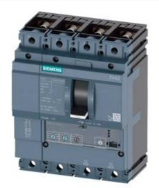
CIRCUIT BREAKER 3VA2 IEC FRAME 100 BREAKING CAPACITY CLASS M ICU=55KA @ 415 V 4POLE, LINE PROTECTION ETU320, LI, IN=40A OVERLOAD PROTECTION IR=16A ...40A SHORT CIRCUIT PROTECTION II=12 X IN NEUTRAL PROTECTION ADJUSTABLE(OFF,100%) BUSBAR CONNECTION
