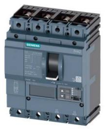
CIRCUIT BREAKER 3VA2 IEC FRAME 160 BREAKING CAPACITY CLASS H ICU=85KA @ 415 V 4POLE, LINE PROTECTION ETU550, LSI, IN=40A OVERLOAD PROTECTION IR=16A ...40A SHORT CIRCUIT PROTECTION ISD=0,6..10X IN, II=1,5..12X IN NEUTRAL PROTECTION ADJUSTABLE (OFF, UPTO 160%) BUSBAR CONNECTION
