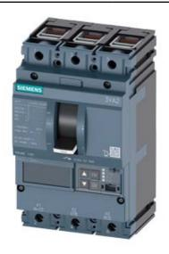
CIRCUIT BREAKER 3VA2 IEC FRAME 160 BREAKING CAPACITY CLASS H ICU=85KA @ 415 V 3POLE, LINE PROTECTION ETU560, LSIG, IN=63A OVERLOAD PROTECTION IR=25A ...63A SHORT CIRCUIT PROTECTION ISD=0,6..10X IN, II=1,5...12X IN NEUTRAL PROTECTION OPTIONAL WITH EXT. CT,UPTO 160% GROUNDFAULT, SWITCHABLE IG=0,2... 1 X IN, TG=0,050,8MS CABLE CONNECTION
