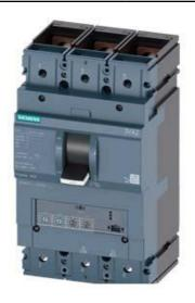
CIRCUIT BREAKER 3VA2 IEC FRAME 400 BREAKING CAPACITY CLASS H ICU=85KA @ 415 V 3-POLE, LINE PROTECTION ETU350, LSI, IN=250A OVERLOAD PROTECTION IR=100A ...250A SHORT CIRCUIT PROTECTION ISD=1,5... 10 X IR, II=12 X IN BUSBAR CONNECTION
