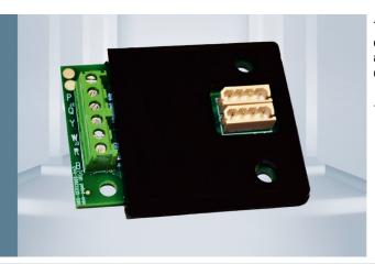
The A2P interface is a 0-10 volt to open collector PWM converter and is designed to work with ebm-papst 4 wire PWM controlled DC fans. The interface translates the analogue voltage input to an equivalent PWM signal. The interface is matched to the fan so that with its very low power consumption, there is no need for a separate dedicated power supply.
