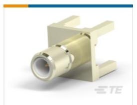
TE Part # CAT-884-SMBV50 SMB Connector: Male (Jack), Vertical Mount, Mated Outer Dia. 4.75mm, 50 Ohm
