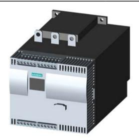
SIRIUS SOFT STARTER, VALUES WITH 400 V, 40 DEG., STANDARD: 162A, 90KW, INSIDE-DELTA CIRCUIT 3: 281A, 160KW, 200-460 V AC, 230 V AC, SCREW TERMINALS
