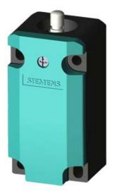
SIRIUS POSITION SWITCH, BASIC SWITCH, METAL, 40MM, ACC.TO EN50041 INCREASED CORROSION PROTECTION, DEVICE CONNECTION 1X (M20X1.5) 1NO/1NC QUICK-ACT.CONTACTS FUNCTIONAL AT -40 DEGREES, SHOCK-AND VIBRATION TEST ACC.TO EN61373, CATEGORY 1B
