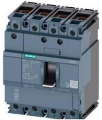
CIRCUIT BREAKER 3VA1 IEC FRAME 160 BREAKING CAPACITY CLASS N ICU=25KA @ 415 V 4-POLE, LINE PROTECTION TM210, FTFM, IN=100A OVERLOAD PROTECTION IR=100A FIXED SHORT CIRCUIT PROTECTION II=10 X IN NEUTRAL UNPROTECTED CABLE CONNECTION
