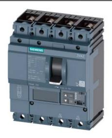
CIRCUIT BREAKER 3VA2 IEC FRAME 250 BREAKING CAPACITY CLASS C ICU=110KA @ 415 V 4POLE, LINE PROTECTION ETU560, LSIG, IN=250A OVERLOAD PROTECTION IR=100A ...250A SHORT CIRCUIT PROTECTION ISD=0,6..10X IN, II=1,5..10X IN NEUTRAL PROTECTION ADJUSTABLE (OFF, UPTO 100%) GROUNDFAULT, SWITCHABLE IG=0,2... 1 X IN, TG=0,050,8MS BUSBAR CONNECTION
