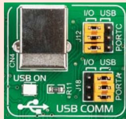
Figure 8-3: USB enabled on PORTA
