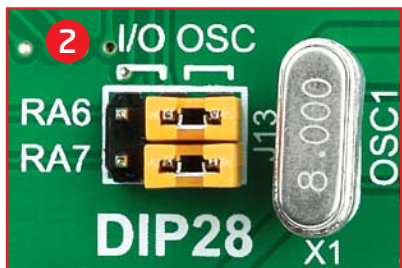
Figure 4-7: RA6 and RA7 connected to X1 quartz-crystal
