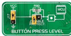
Figure 10-5: Button press level jumper (J17)
