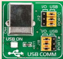
Figure 8-2: USB enabled on PORTC
