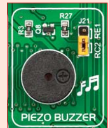
Figure 19-2: Use jumper J21 to connect Piezo buzzer on RE1 or RC2 pin
