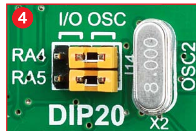
Figure 4-9: RA4 and RA5 connected to X2 quartz-crystal
