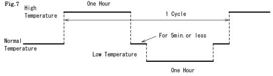
Termostatic chamber temperature is set at 125°C as the high temperature and -40°C as the low temperature
