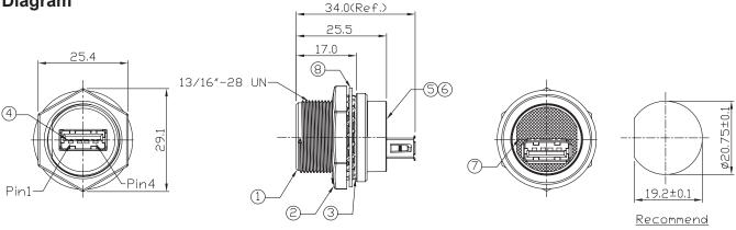
Panel Cut-Out Dimensions: Millimetres
