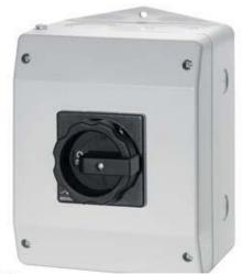
MAIN CONTROL SWITCH 4-POLE IU=25, P/AC-23A AT 400V=9,5KW 1 N-TERMINAL ENCAPSUL.IN M.P.ENCLOSURE, IP65 ROTARY ACTUATOR BLACK METRIC THREAD
