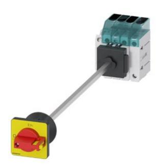
Switch disconnector 3LD3, main switch 3-polig + N, lu 32A operational switch at AC-23 A at 400 V 11,5 kW floor mounting Base mounting with door coupling center-hole 22,5 mm knob-operated mechanism red/yellow 48 x 48 mm with auxiliary 1NO+1NC
