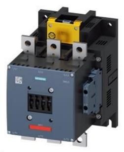
Contactor AC3: 160kW / 400 V 3-pole Size S10 Coil AC 50/60Hz and DC 200...277 V x (0,8...1,1) auxiliary contacts: 2 NO + 2 NC permanently mounted (SUVA) Main: busbar connections coil and auxilliary: screw terminal
