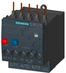
OVERLOAD RELAY 0.18...0.25 A FOR MOTOR PROTECTION SZ S00, CLASS 10, F. MOUNTING ONTO CONTACTOR MAIN CIRCUIT: SCREW TERMINAL AUX. CIRCUIT: SCREW TERMINAL MANUAL-AUTOMATIC-RESET
