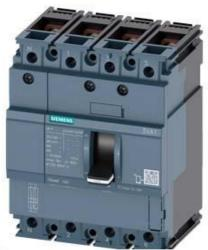
CIRCUIT BREAKER 3VA1 IEC FRAME 160 BREAKING CAPACITY CLASS S ICU=36KA @ 415 V 4-POLE, LINE PROTECTION TM210, FTFM, IN=160A OVERLOAD PROTECTION IR=160A FIXED SHORT CIRCUIT PROTECTION II=10 X IN NEUTRAL UNPROTECTED BUSBAR CONNECTION
