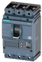
CIRCUIT BREAKER 3VA2 IEC FRAME 160 BREAKING CAPACITY CLASS L ICU=150KA @ 415 V 3POLE, LINE PROTECTION ETU550, LSI, IN=160A OVERLOAD PROTECTION IR=64A ...160A SHORT CIRCUIT PROTECTION ISD=0,6..10X IN, II=1,5..10X IN NEUTRAL PROTECTION OPTIONAL WITH EXT. CT,UPTO 160% BUSBAR CONNECTION
