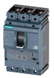
CIRCUIT BREAKER 3VA2 IEC FRAME 160 BREAKING CAPACITY CLASS L ICU=150KA @ 415 V 3POLE, LINE PROTECTION ETU330, LIG, IN=40A OVERLOAD PROTECTION IR=16A ...40A SHORT CIRCUIT PROTECTION II=1,5...12 X IN GROUNDFAULTPROTECTION IG=0,2... 1 X IN, TG=0,1/0,3MS BUSBAR CONNECTION
