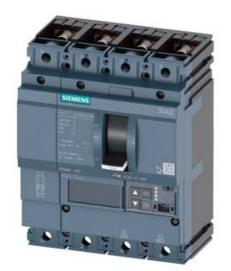
CIRCUIT BREAKER 3VA2 IEC FRAME 160 BREAKING CAPACITY CLASS C ICU=110KA @ 415 V 4POLE, LINE PROTECTION ETU850, LSI, IN=63A OVERLOAD PROTECTION IR=25A ...63A SHORT CIRCUIT PROTECTION ISD=0,6..10X IN, II=1,5..12X IN NEUTRAL PROTECTION ADJUSTABLE (OFF, UPTO 160%) BUSBAR CONNECTION
