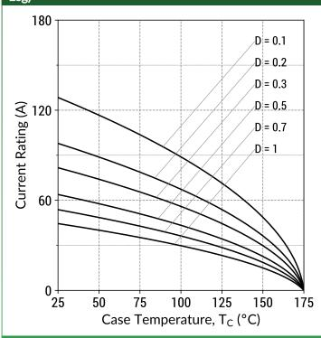
$I_F = f(T_C); D = t_P/T; T_j \le 175^{\circ}C; f_{SW} > 10kHz$
