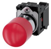
EMERGENCY STOP mushroom pushbutton, 22 mm, round, metal, shiny, red, 30 mm, positive latching, according to DIN EN ISO 13850, rotate-to-unlatch, washer for EMERGENCY STOP, yellow, without inscription, with holder, 1 NC, springloaded terminal, front plate mounting
