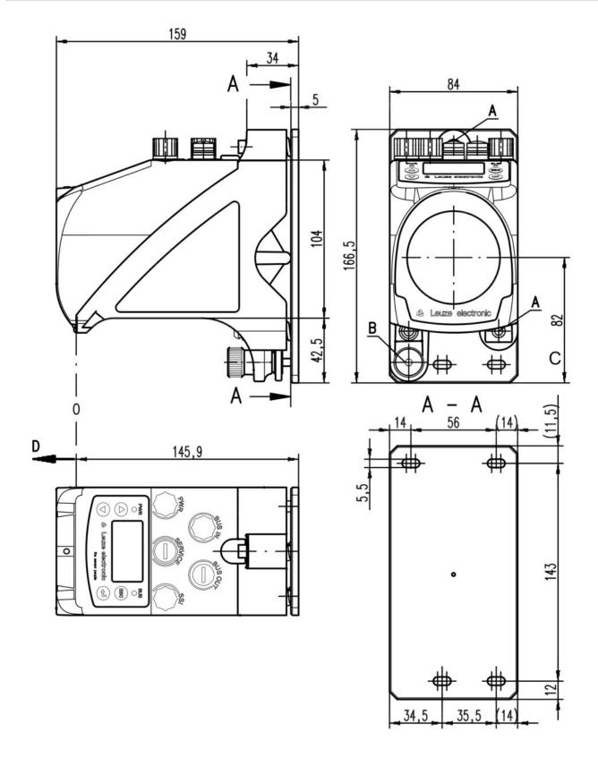
A M 5 screw for alignment B Knurled nut with WAF 4 hexagon socket and M 5 nut for securing
