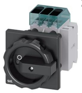
Switch disconnector 3LD3, main switch 3-polig, lu 25A operational switch at AC-23 A at 400 V 9,0 kW front mounted Base mounting with center-hole 22,5 mm knob-operated mechanism black 66 x66 mm with auxiliary 1NO+1NC
