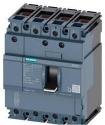
CIRCUIT BREAKER 3VA1 IEC FRAME 160 BREAKING CAPACITY CLASS S ICU=36KA @ 415 V 4-POLE, LINE PROTECTION TM210, FTFM, IN=63A OVERLOAD PROTECTION IR=63A FIXED SHORT CIRCUIT PROTECTION II=10 X IN NEUTRAL UNPROTECTED CABLE CONNECTION
