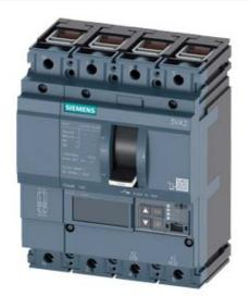
CIRCUIT BREAKER 3VA2 IEC FRAME 160 BREAKING CAPACITY CLASS C ICU=110KA @ 415 V 4POLE, LINE PROTECTION ETU560, LSIG, IN=160A OVERLOAD PROTECTION IR=64A ...160A SHORT CIRCUIT PROTECTION ISD=0,6..10X IN, II=1,5..10X IN NEUTRAL PROTECTION ADJUSTABLE (OFF, UPTO 100%) GROUNDFAULT, SWITCHABLE IG=0,2... 1 X IN, TG=0,050,8MS CABLE CONNECTION
