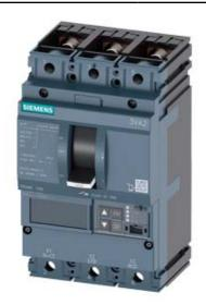
CIRCUIT BREAKER 3VA2 IEC FRAME 160 BREAKING CAPACITY CLASS M ICU=55KA @ 415 V 3POLE, LINE PROTECTION ETU860, LSIG, IN=25A OVERLOAD PROTECTION IR=10A ...25A SHORT CIRCUIT PROTECTION ISD=0,6..10X IN, II=1,5..12X IN NEUTRAL PROTECTION OPTIONAL WITH EXT. CT,UPTO 160% GROUNDFAULT, SWITCHABLE IG=0,2... 1 X IN, TG=0,050,8MS BUSBAR CONNECTION
