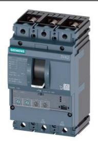
CIRCUIT BREAKER 3VA2 IEC FRAME 160 BREAKING CAPACITY CLASS L ICU=150KA @ 415 V 3POLE, LINE PROTECTION ETU330, LIG, IN=25A OVERLOAD PROTECTION IR=10A ...25A SHORT CIRCUIT PROTECTION II=1,5...12 X IN GROUNDFAULTPROTECTION IG=0,2... 1 X IN, TG=0,1/0,3MS BUSBAR CONNECTION
