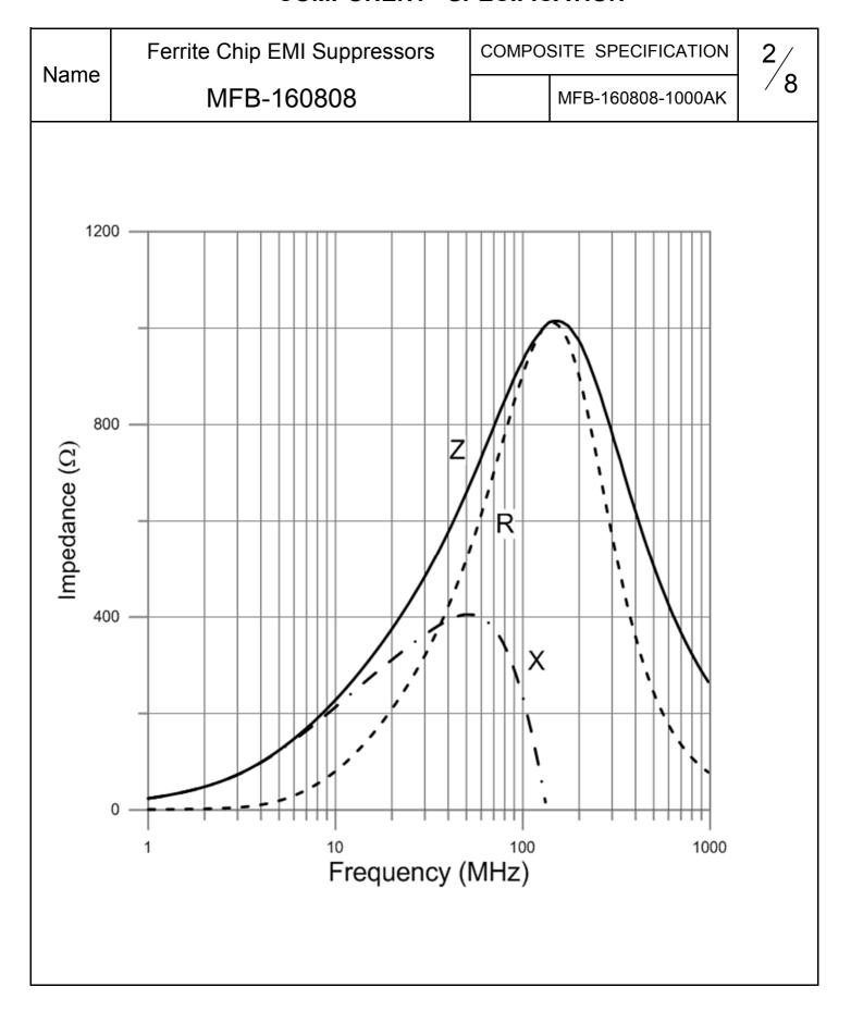
Ferrite Chip EMI Suppressors COMPOSITE SPECIFICATION Name MFB-160808 MFB-160808-1000AK
