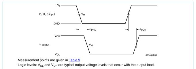
Fig. 6. The data inputs (I0, I1) and common data select input (S) to output (Y) propagation delays
