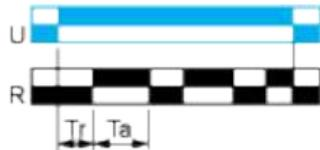
Function Li : Asymmetrical Flasher Relay (Starting Pulse On)
