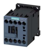
Contactor relay, 3 NO + 1 NC, 240 V AC, 50 / 60 Hz, Size S00, screw terminal
