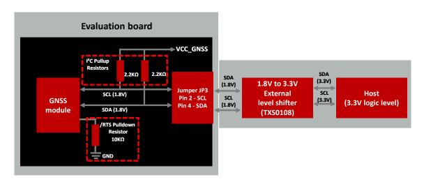
Figure 14: I<sup>2</sup>C Hardware setup - Erinome-II
