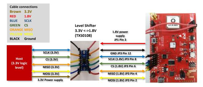
Figure 19: SPI communication setup - Erinome-II evaluation board to 3.3V Host
