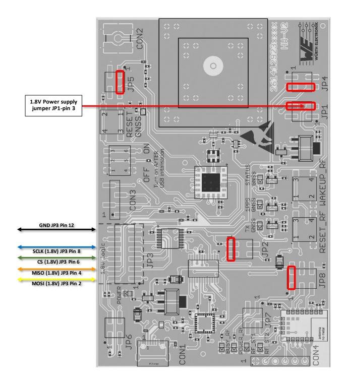
Figure 18: SPI bus access on evaluation board
