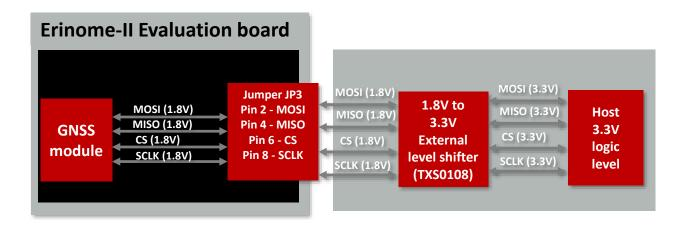
Figure 17: SPI Hardware setup
