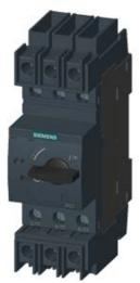
CIRCUIT-BREAKER SZ S00, FOR TRANSFORMER PROTECTION, WITH APPROBATION CIRCUIT-BREAKER UL 489. CSA C22.2 NO.5-02. A-RELEASE 4 A, N-RELEASE 82 A, SCREW CONNECTION, STANDARD SW. CAPACITY
