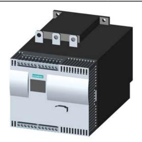
SIRIUS SOFT STARTER, VALUES WITH 400 V, 40 DEG., STANDARD: 134A, 75KW, INSIDE-DELTA CIRCUIT 3: 232A, 132KW, 200-460 V AC, 230 V AC, SCREW TERMINALS
