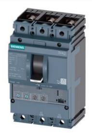
CIRCUIT BREAKER 3VA2 IEC FRAME 160 BREAKING CAPACITY CLASS C ICU=110KA @ 415 V 3POLE, LINE PROTECTION ETU350, LSI, IN=25A OVERLOAD PROTECTION IR=10A ...25A SHORT CIRCUIT PROTECTION ISD=1,5... 10 X IR, II=12 X IN BUSBAR CONNECTION
