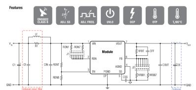
The additional aluminium electrolytic capacitor C1 is only for evaluation board protection purposes. It is mounted at the termination of the supply line and provides slight damping of possible oscillations of the series resonance circuit represented by the inductance of the supply line and the input capacitance. It is not essential for operation. The switching frequency of the module can be additsted by changing the position of jumper J1.
